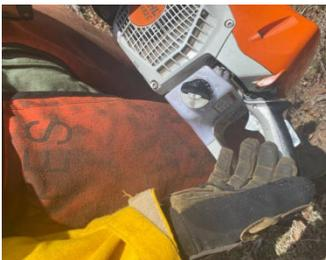
**Brushing Project - 2020** Suspicious of a vapor-lock, he set the saw aside for continued cooling. Several minutes later, the sawyer cautiously opened the saw’s fuel tank – a geyser occurred. Sawyer had anticipated the geyser and was able to reduce the volatility by careful placement of his hand over the fuel cap as he opened it. Even so, this incident still resulted in his (gloved) hand and chaps becoming soaked in saw gas.
